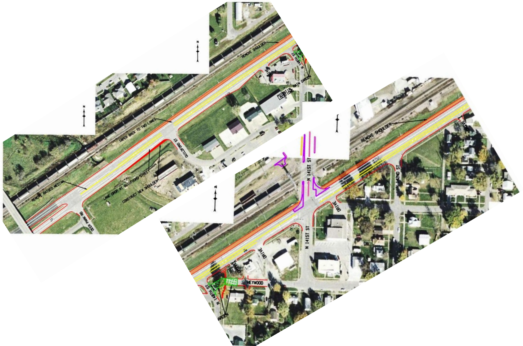
Figure T- 5.1. US Highway 6 Three-Lane Conceptual Plan
